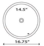
Drain Hole Diameter 1.75" Standard Vanity Drain Required With Overflow
