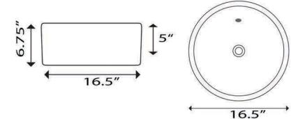
Drain Hole Diameter 1.75" Standard Vanity Drain Required With Overflow
